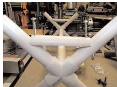
Once you have these placed, it's time to put the pipe-insulation foam in to hold the airplane in place. Cut the foam to fit your cradle, and place it on top of the cradle as shown in the picture. You can either glue it in place or put tie wraps at the ends. Now it's all done!
