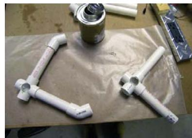
Take the 21.25-inch pipe and insert it into the hole that you drilled in one of the crosses. Gluing this piece is optional dependent on how snug the fit is.
