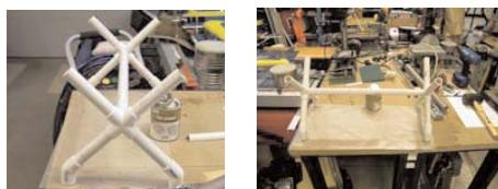
Now take the 4.5-inch sections of pipe and center them into the top of the crosses. Drill a hole on each side to fit your screws and screw them into place. Do not tighten too much; snug is just right.
