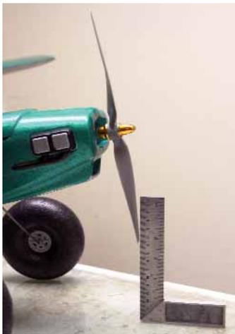
We all know it is imperative to balance a propeller before installing it on your airplane. It is also important to check propeller tracking whenever installing a new propeller. A propeller that is not tracking properly will cause vibration similar to that of an out-of-balance propeller.
