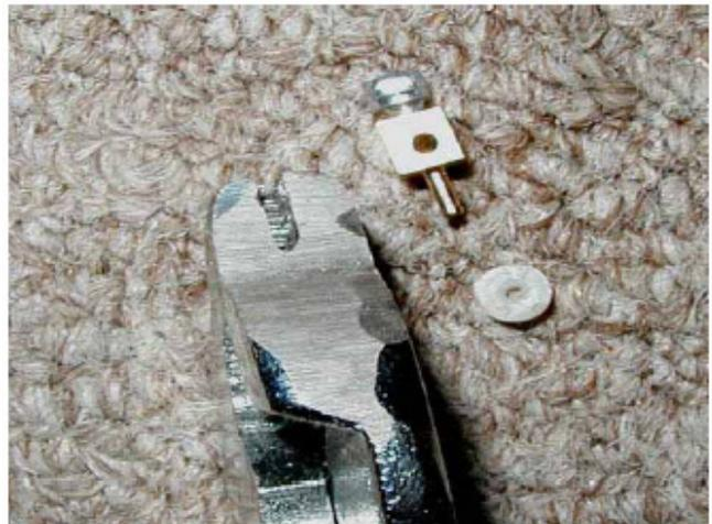
I hope this image shows up enough? In any event, I was having a problem attaching those " quick connectors" to servo arms so I went to the dollar store and bought a pair of slip joint pliers and ground the outside of the pliers sorta flat and then took my trusty Dremel® motor tool with the grinding wheel disk and cut a slot in one of the jaws that the stem of the connector will pass through. Works like a charm as the old saying goes.
