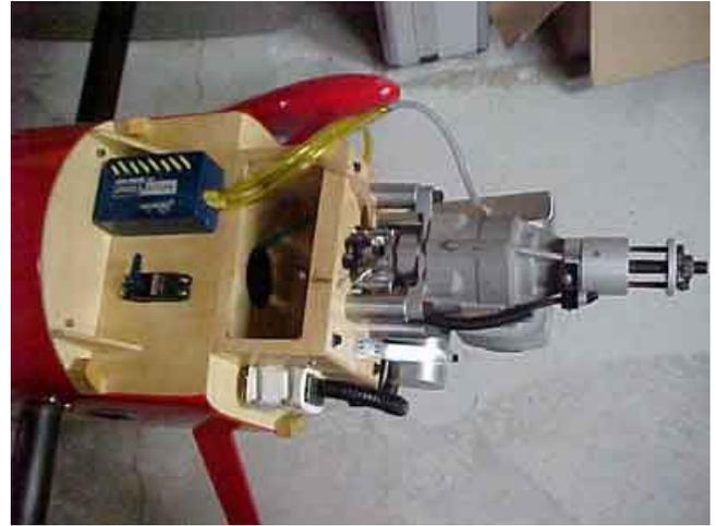
Batteries and switches would all have to be installed as far forward as I could get them. I did not want to add any "dead weight" to the front of the plane to get the plane to balance out. I even went as far as cutting about 6oz out of the canopy/hatch area to loose some of the aft CG weight. The fuel tanks were moved from the front of the plane to over the wing tube to minimize in-flight changing CG.
