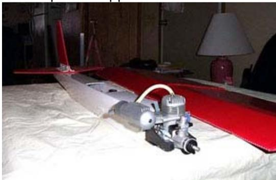
Its not completely finished yet, I still have to finish mounting the radio gear and the wing servo/rods, balance the wing and drill the dowel rod holes to mount the wing. I may also put a gear on it as well, haven't decided yet. I hooked my old 40 LA up for a motor and figure on make up for the low power with prop size (11x4).
