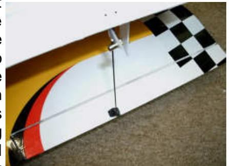
a cut up horn from my stash so I could get the right mechanical linkage set up.
