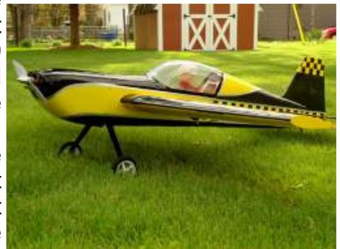
The wings give it lift, the 2826-4T outrunner provides the power, all the control surfaces move in the right direction and the CG is right.
