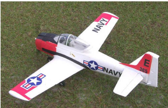
cause I took a turn to fast and didn't have the box tied down. It bent one aileron and one side of the horizontal stabilizer. The aileron bent right back into shape and the stab did too but I stuck some fiberglass backed tape to both sides of the stab for stiffeners just in case. Good as new.
