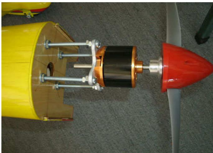
lem? I chose to use 3 inch long 10 X 32 machine screws and enough nuts, T-nuts, flat washers and lock washers to make an adjustable mount with the results shown in the photo.
