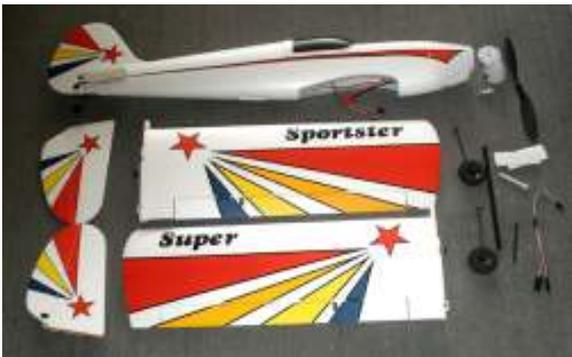
The specs on the plane: wingspan 40 inches, length 32.5 inches, wing area 267 sq inches, weight 20-22 ounces and a wing loading of 10.8 to 11.5 oz/sq foot. Close to those of the T-28.
