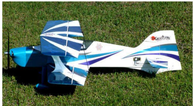
The Reactor Bipe has a 35 inch wingspan and the fuse is about 44 inches long and it fits in the van nicely and that's a good thing because the instruction manual has you gluing the wings and tail feathers on so about the only thing you can take apart on the plane is the landing gear and the prop.
