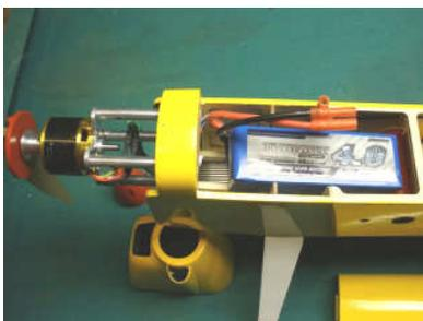
The engine cowl was the easiest I have ever mounted with no muffler, no needle valve, or fuel line holes to mess with. A much cleaner look. I added lots of air-flow opening to the front, just as any other engine would require.
