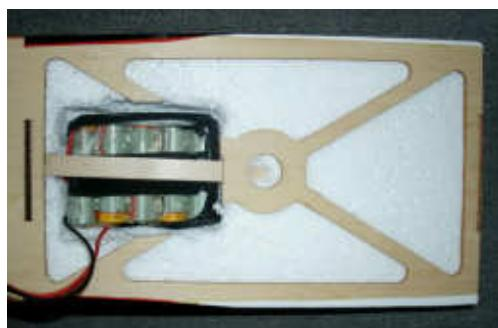
ward fuselage and mount the battery so. Now the planes C/G was on the money with either 6 cell Li-Po I have. One is about one inch longer then the other and doesn't give me any "wiggle room" to move back and forth.
