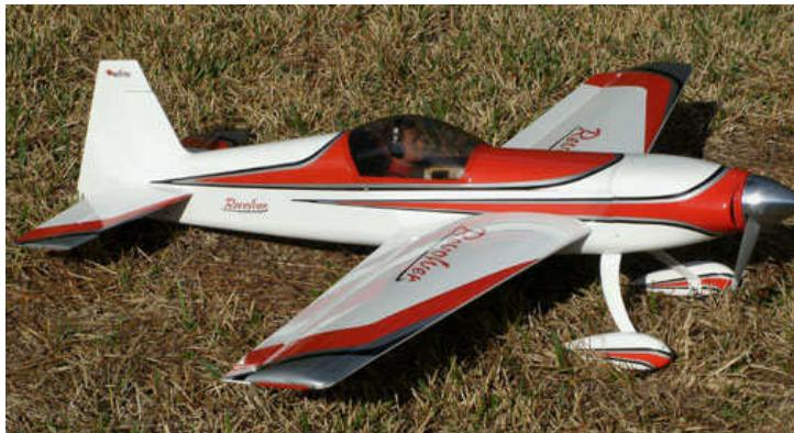
I've started out the new year with a new plane, the Great Planes Revolver. The plane has a 59 inch wingspan and weighs 6-7 pounds with a wing loading of 25-29 oz/ft<sup>2</sup> so it should fly fine. I'll let you know on page two after the first of ,many I hope, flights.
