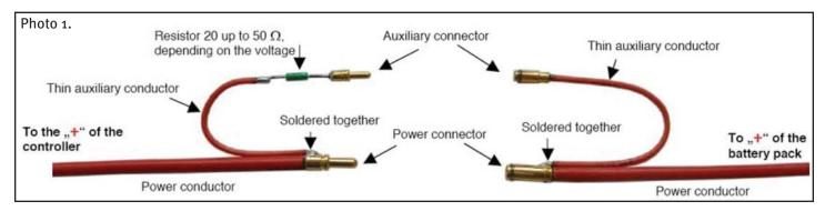
When connecting a LiPo pack to the controller, strong sparking commonly occurs. Fast charging of the controller filter capacitors causes this.
