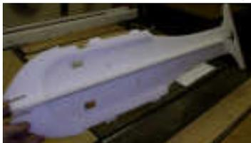
laser cut pieces of light ply glued together and inserted into the fuselage. For the neutral thrust I balanced the plane on its nose and checked the body for square.
