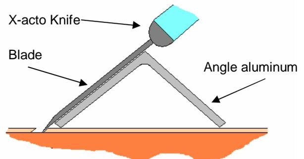
**Cut a perfect bevel** 45 degree with an X-acto knife and a piece of 3/4 X 3/4 angle aluminum, laid on its side. Hold the blade parallel with the aluminum and cut away.
