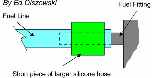
**Silicone fuel line clamp.** A short piece of larger diameter silicone tubing will act like a rubber hose clamp, holding your fuel line in place. Before fitting the fuel line on, use a pair of needle nose pliers to stretch open the piece larger diameter silicone fuel hose over the ends of your fuel line, then push it on to the fittings. The extra friction will hold it in place securely.
