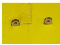
On the left you see the light ply brackets for the wing struts. Two struts and eight ply brackets. Since I have already broken three brackets off at the wing surface I
