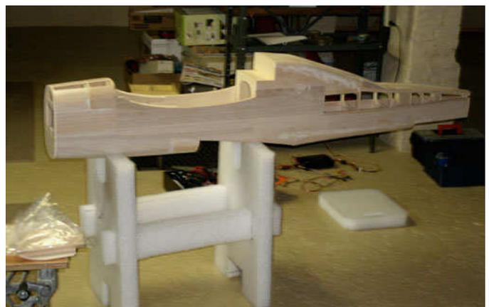
I'm this far along and decided to leave some skin off of the fuse because I'll mount the elevator and rudder servos in the back. No long dowels, eh!
