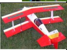
**Great planes extra 300 40** with Super Tiger G51 ringed engine, Futaba s3003 throttle, futaba s3004 elevator, MPI on off charge switch with voltage indicator built in.
