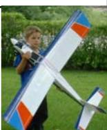
**Dave Patrick Ultimate 40** ready to fly with an O.S.50 SX, Tower ts 35 servos, receiver, 1100ma. 6v. battery, MPI volt meter. The plane is in good condition but has not flown in 2 years.
