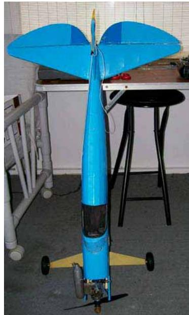
I used a hack saw and sawed half way through the fuse just behind the cockpit on the right side so I would have wood on either side of the cut and used popcycle stick pieces and pulled the gap together and "hot stuffed" the thing back together and that got out most of the curve. The vertical stab stayed pretty much in line and the "fix" proved out because that Whimpy II flies pretty nice.
